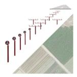
Medium Intensity Approach Lighting System with Runway Alignment Indicator Lights
