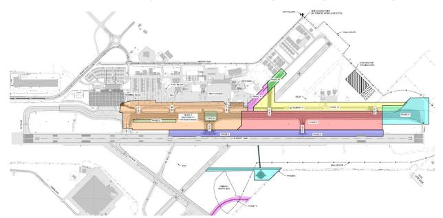
work will involve clearing and grubbing, grading, pavement removal and replacement, edge lighting, utility and storm drainage improvements, airfield signage, and pavement markings. The current engineer's estimate, provided by TO Engineers, is \$17.6 million. The Airport has applied for FAA grant funds which will fund 90% of the project, and if successful, work will begin in August 2022 and be completed in 2023.
